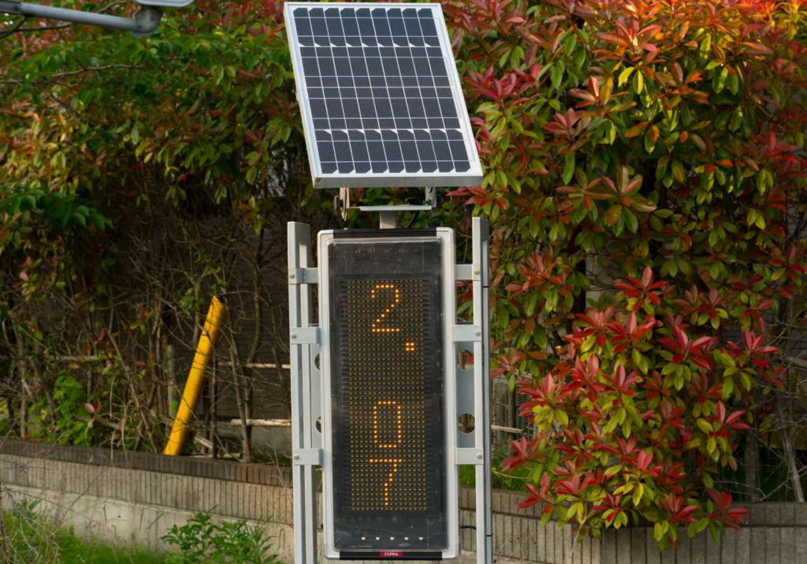
Radiations sensors indicate the level of radioactivity, but in these red zones classified as "difficulty to return to zones" by the government, no one is there to read them. 1 millisievert is the maximum radiation dose allowed for Japanese per year.
